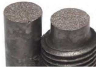
(b) Brittle fracture in a mild steel.
