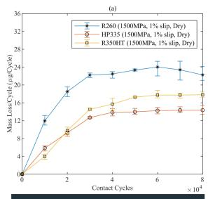
Twin disc data showing lower wear rate for HP335 than R350HT
