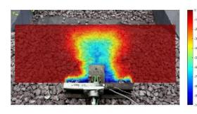
Premium rails are not the only product requiring validation data to aid adoption: we have developed a custom test rig to show steel sleepers can provide excellent lateral resistance.
