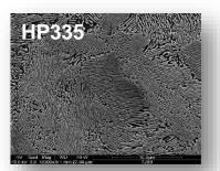
HP335 is an as-rolled premium rail steel, getting its strength from metallurgical engineering rather than heat treatment
