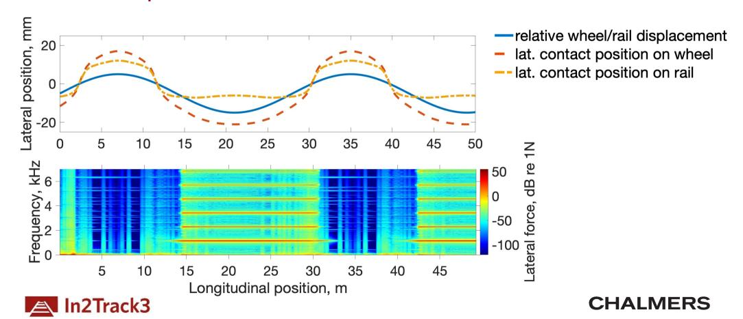
Sinusoidal path of the wheelset on the rail
